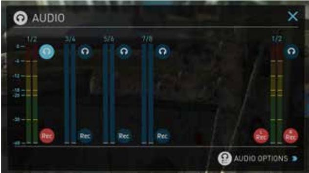
Each channel has a level meter assigned to Left & Right Channels; when there is active audio feed you will see the level indicator moving.
