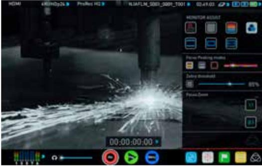
Blue only displays a greyscale image based on the blue channel of the input signal. This is useful to observe the noise content of a video image as sensor noise is most visible in this channel.
