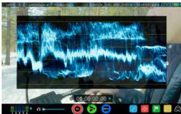
The Luma or Luminance Waveform is a great way to visualize the dynamic range of your image, allowing you to protect exposure of both your high lights and shadow detail. It's particularly useful when shooting with a low contrast LOG curve and works in perfect partnership with the AtomHDR engine to illustrate the highlight clipping point to allow you to correctly expose your image.
