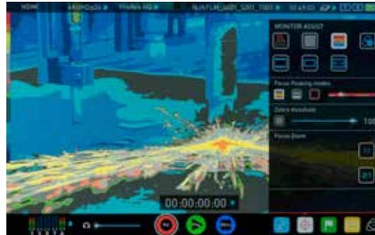
False Colour assigns different colors to areas of different brightness in the image. This gives a visualization of what is going on with exposure across the image. There is a scale on the left hand side, overexposed elements will display as red, and underexposed elements will display as blue.
