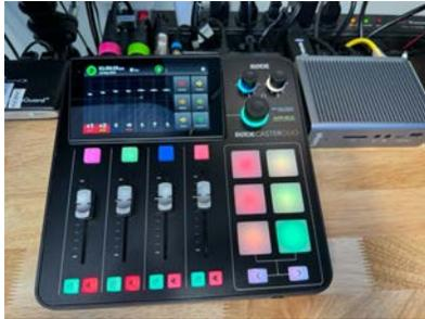
The audio is controlled by the RØDEcaster Duo device. If the device is off, turn it on by pressing the red power button on the back.
