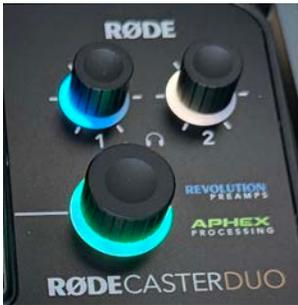
The output controls for the headphones and the speakers are located at the top-right of the unit.
