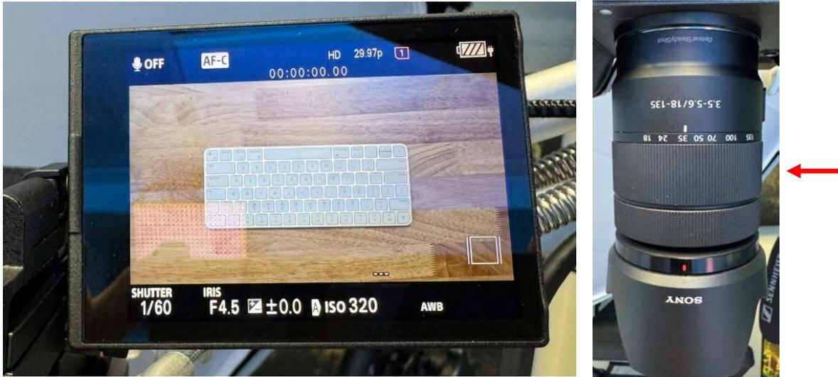
10. Ensure that the overhead camera is high enough and doesn't show on the teleprompter screen in the front-facing camera frame.
