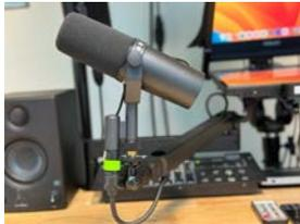
Use the **Shure SM7B** microphone to record videos with the microphone in front of you. This industry-standard microphone for podcasting and broadcasting captures a flat "radio" voice. It is connected to Input 2 of the RØDECaster Duo and is color-coded green. The microphone should be placed 1-6 inches from your mouth.
