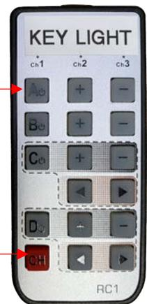
Alternatively, you can press the power button on the controller hanging on the light stand beneath the light.
