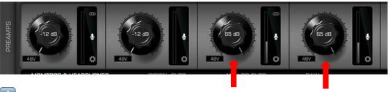
Note that for the additional studio mics (Shure SM57, SM58, and Beta58A) used with input 1 and input 2, the gain level of about 45 dB is sufficient.
