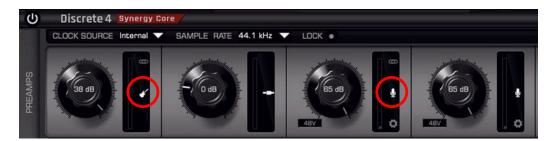
6. The two microphones (Shure SM7B) mounted on two arms are connected to **input 3** and **input 4** on the back of the console. Ensure that the gain of these mics is at <u>60-65 dB</u>:
