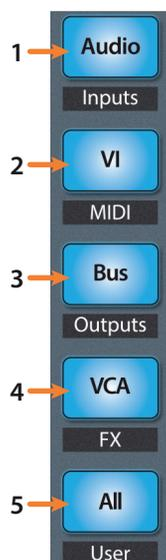
1. **Audio / Inputs.** Press to view Audio tracks only. Press Shift + Audio to create a new audio channel.
