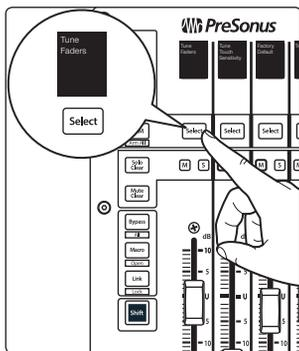
To adjust your fader speed, press the Select button beneath the Tune Faders screen. This will open the Tune Faders menu.
