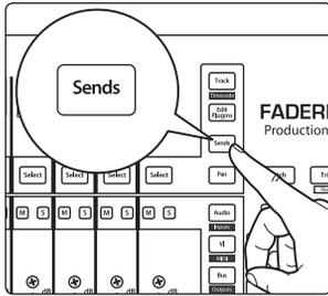
Pressing Sends allows you to edit the assigned bus sends for the currently selected channel.
