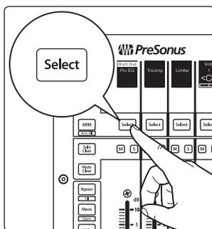
2. Press the Select button under the scribble strip displaying the name of the plug-in you'd like to edit.
