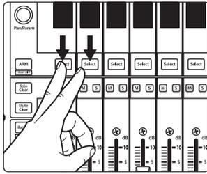
By default, the operation mode on the FaderPort is set Studio One. To switch to Logic operation, power on the unit while pressing the first two select buttons.
