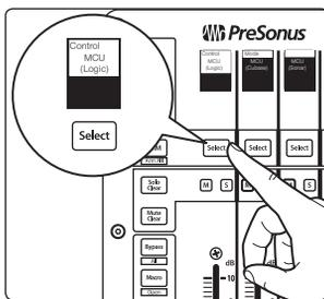
When using the FaderPort with Logic, select MCU (Logic) by pressing the Select button below its scribble strip.
