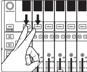
If you have changed the FaderPort's Operating Mode and would like to return to using it with Studio One, press the first two Select buttons while powering on your unit.
