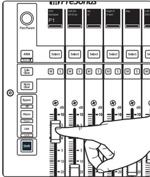
4. This displays the plug-in parameters on the scribble strips and allows you to control each parameter with the corresponding fader. Use the Pan/Param encoder to scroll through other plugins on the same channel.
