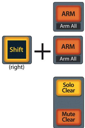
**ARM.** Pressing the Arm button will allow you to arm track for recording by pressing the corresponding track's Select button.
