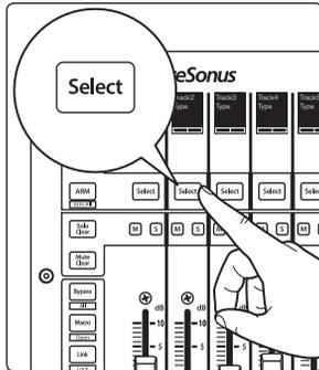
Press the Select button below any of the insert slots to enable or disable that plug-in.
