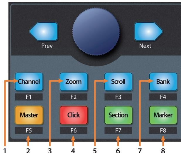
1. **Channel.** Encoder scrolls and selects individual channels. Navigation buttons adjust the current bank by one channel.
