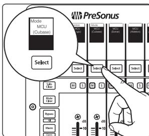
When using the FaderPort with Cubase, select MCU (Cubase) by pressing the Select button below its scribble strip.
