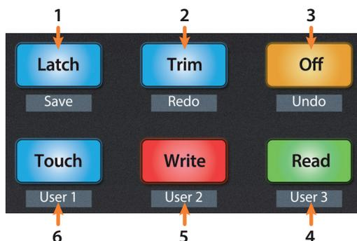
1. **Latch / Save.** Engages Latch Automation on currently selected track. Press the SHIFT and Latch buttons twice simultaneously to save your session.
