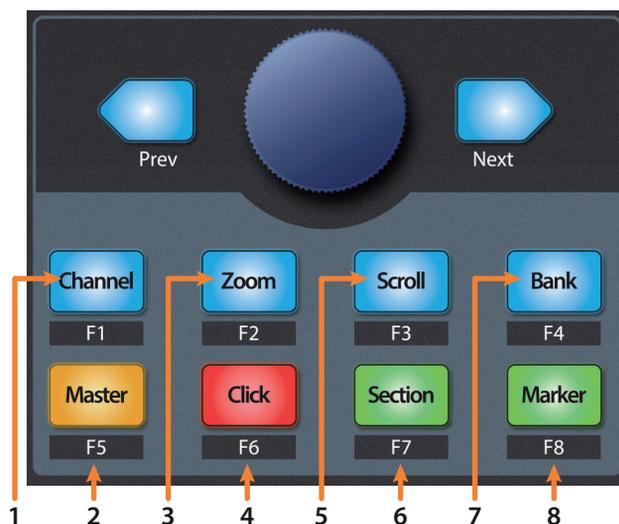
1. **Channel.** Encoder and navigation buttons adjust the currently visible fader bank on the FaderPort by one channel. Press Shift and Channel to clear clip and peak holds.
