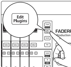
1. Press Edit Plug-ins twice. This will display every insert slot for the currently selected channel in the scribble strips.
