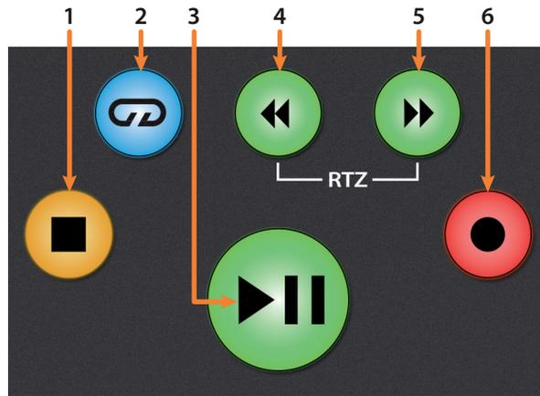
1. **Stop.** Stops playback. Press twice to return to the initial playback position.
