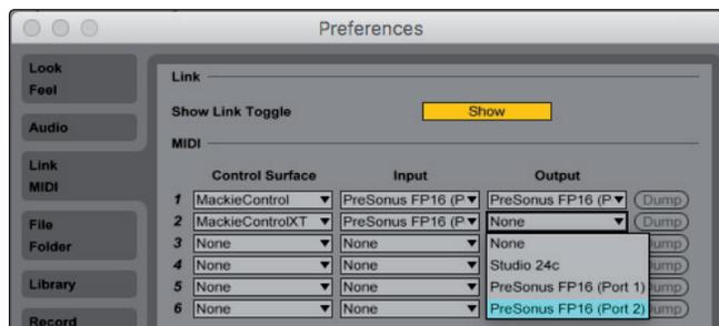
5. Make sure that Track, Sync, and Remote are all enabled for both the Input and the Output for both devices.
