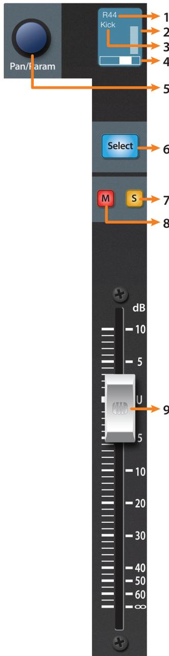
1. **Pan Value.** Displays Pan Value while panning is actively being adjusted.
