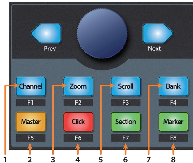
1. **Channel.** Encoder controls individual channel scrolling. Navigation buttons adjust the currently visible fader bank on the FaderPort by one channel.
