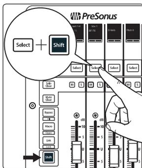
2. Press SHIFT with the Select button for the channel you'd like view.
