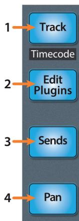
1. **Track.** When Track mode is active, the motorized faders will display and control channel levels. Press Shift and Track simultaneously to display Timecode on the scribble strips. *See Section 6.6.3 for more information.*
