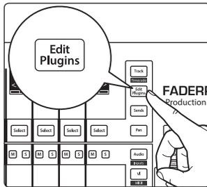
Pressing Edit Plug-ins will allow you to view and edit the insert slots for the currently selected channel. While active:
