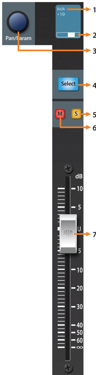
1. **Channel Name.** Displays the Channel name and current fader level when a fader is touched.
