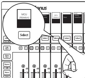
When using the FaderPort with Live, select MCU (Ableton) by pressing the Select button below its scribble strip.
