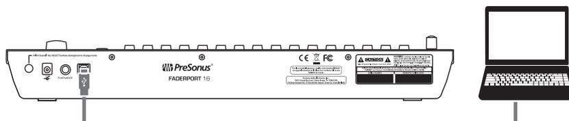
Once you have connected your FaderPort to your computer, launch Pro Tools to set up the FaderPort as a HUI device. The FaderPort 16 requires that you configure it as two HUI devices, while the FaderPort 8 only requires you to configure it as a single HUI device.
