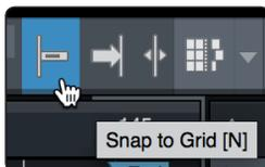
**Power User Tip:** Enable Snap to Grid for coarse nudging. Disable it for fine tuning. By default, this button is controlled by the User 2 function on the FaderPort. See Section 2.5.1 for details.
