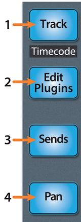
1. **Track.** When Track mode is active, the motorized faders will display and control channel levels. Press Shift and Track simultaneously to display Timecode on the scribble strips. *See Section 4.6.2 for more information.*
