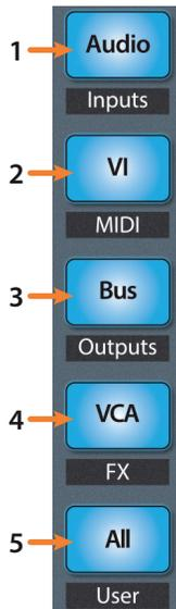
1. **Audio / Inputs.** Press to view Audio tracks only. Press Shift + Audio to view all Input channels.
