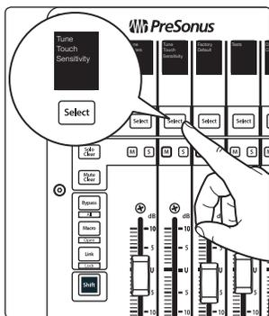
To adjust the touch sensitivity of your faders, press the Select button beneath the Tune Fader Sensitivity screen. This will open the Fader Sensitivity menu.
