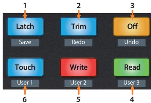
1. **Latch / Save.** Press the SHIFT and Latch buttons simultaneously to save session. At the time of publication, Latch automation control is not available in Sonar.
