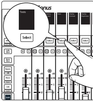
Your FaderPort is equipped with multiple test modes to verify electrical functionality of all its components. Press the Select button below the Test screen to access these modes.
