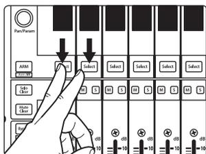
By default, the FaderPort is in Studio One operation mode. To switch to Pro Tools operation, power on the unit while pressing the first two select buttons.
