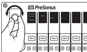
Turn the Pan/Param encoder on the left until the desired setting has been reached.
