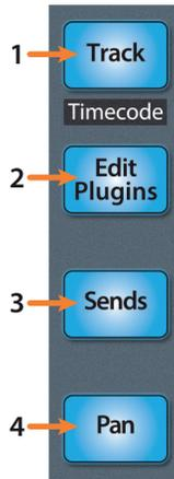
1. **Track.** When Track mode is active, the motorized faders will display and control channel levels. Press Shift and Track simultaneously to display Timecode on the scribble strips. *See Section 5.6.2 for more information.*
