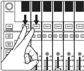
The default operation mode for the FaderPort is Studio One. To switch to Sonar operation, power on the unit while pressing the first two select buttons.
