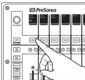
2. Press the Select button below any of the insert slots to edit that plug-in's parameters. Use the Navigation buttons to access additional parameters.
