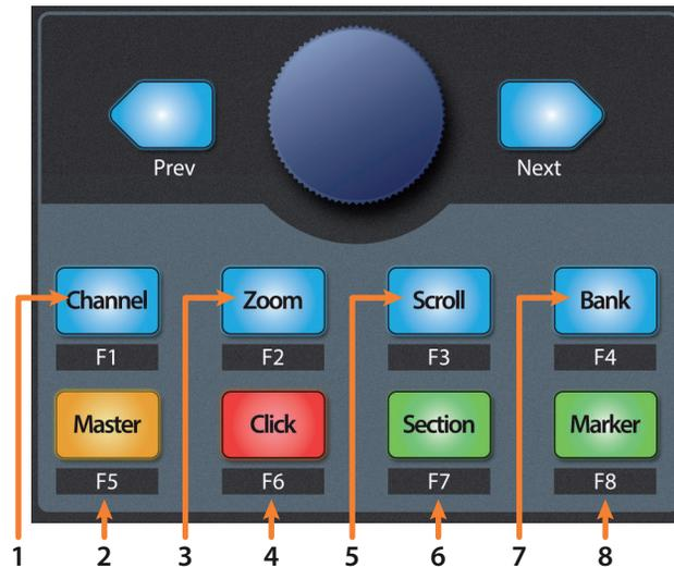
1. **Channel.** Encoder and navigation buttons scroll and select individual channels.
