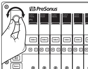
2. Use the Pan/Param encoder to scroll through the available slots. The slot position will be displayed in the lower left-hand corner of the first scribble strip display.
