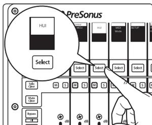
This will open the boot mode screen, and you will be given the opportunity to select which mode of operation you'd like to use. When using the FaderPort with Pro Tools, select HUI by pressing the Select button below its scribble strip.
