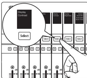
Press the Select button below “Display Contrast” to set the contrast of the scribble strip displays to your desired setting.
