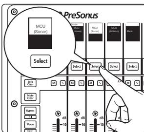
When using the FaderPort with Sonar, select MCU (Sonar) by pressing the Select button below its scribble strip.
