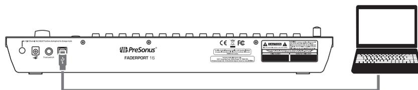
Once you have connected your FaderPort to your computer, launch Logic. The FaderPort 16 will auto-configure as two devices: a Mackie Control Universal and a Mackie Control Extender. The FaderPort 8 will auto-configure as a Mackie Control Universal device only. If for some reason this does not happen, you will need to enable it manually.
