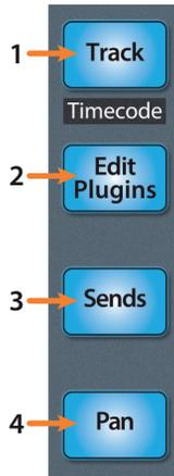
1. **Track.** When Track mode is active, the motorized faders will display and control channel levels. Pressing the Track mode button toggles metering on the scribble strip displays on and off. Press Shift and Track simultaneously to display Timecode on the scribble strips. While Timecode is active, the faders still control level.
