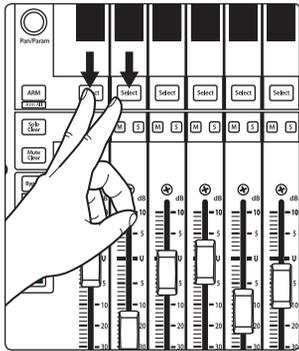
To access this mode, press the first two Select buttons while powering on the FaderPort.
