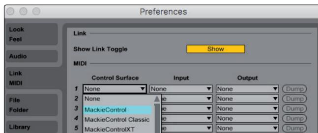
3. Make sure that Track, Sync, and Remote are all enabled for both the Input and the Output of "MackieControl."
