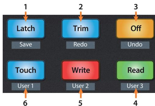
1. **Latch / Save.** Engages Latch Automation on currently selected track. Press the SHIFT and Latch buttons simultaneously to save your session.
